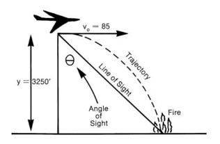
Calculate the angle of sight  $\Theta$  that chemical retardant should be dropped from a fire-fighting plane to reach the fire if the plane is at 3250 feet with a velocity of 85 mph? Using the formula:
